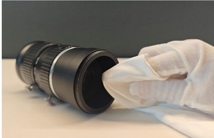
Figure 2-3 Cleaning by Lens Cleaning Paper
