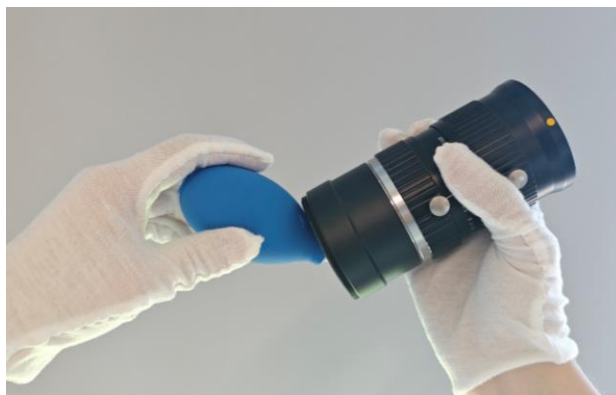
Figure 2-1 Cleaning by Rubber Dust Air Blower
